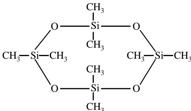
**Figure 3. Chemical Structure for a Siloxane (D4) Molecule**
