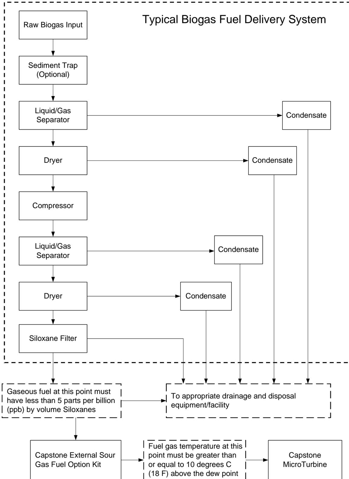
**Figure 1. Typical Flowsheet for Biogas Fuel Delivery System**
